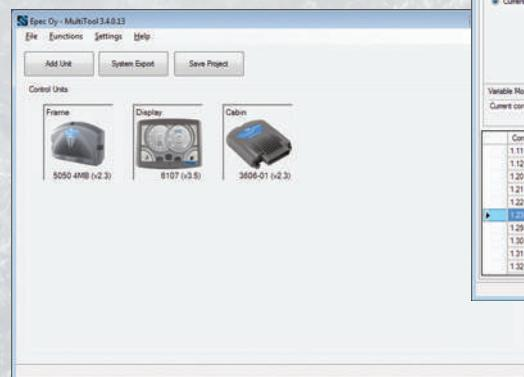
MultiTool supports CODESYS versions 2.3 and/or 3.5 depending on the control units used in the system.
